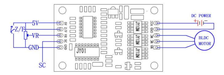
5V -----Driver board internal output voltage
